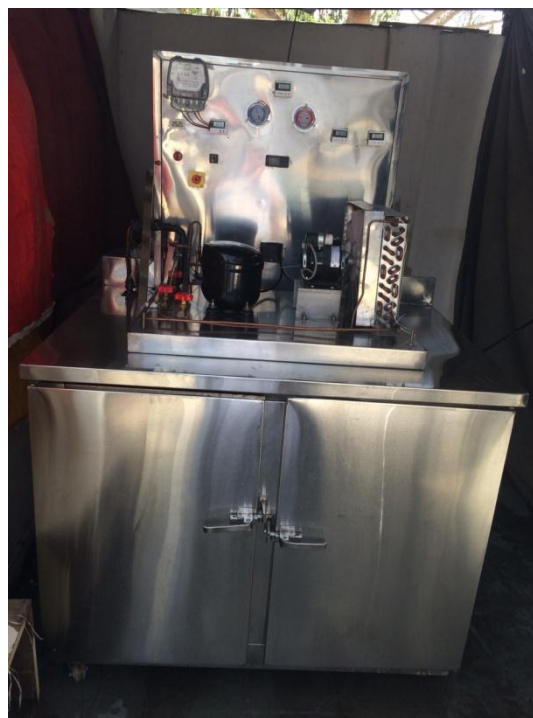
Figure 3: Actual Test Setup of Vapour Compression Refrigeration Deep Freezer.
