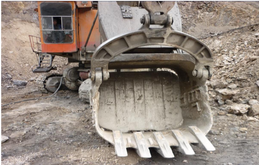
Fig. 3: General view of the front wall of the bucket with established teeth on it.
