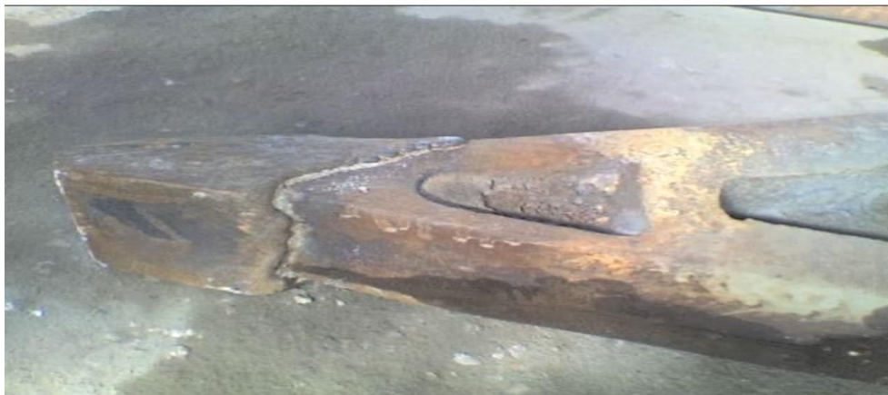
Fig. 2: General view of the teeth of steel welds 50HG.
