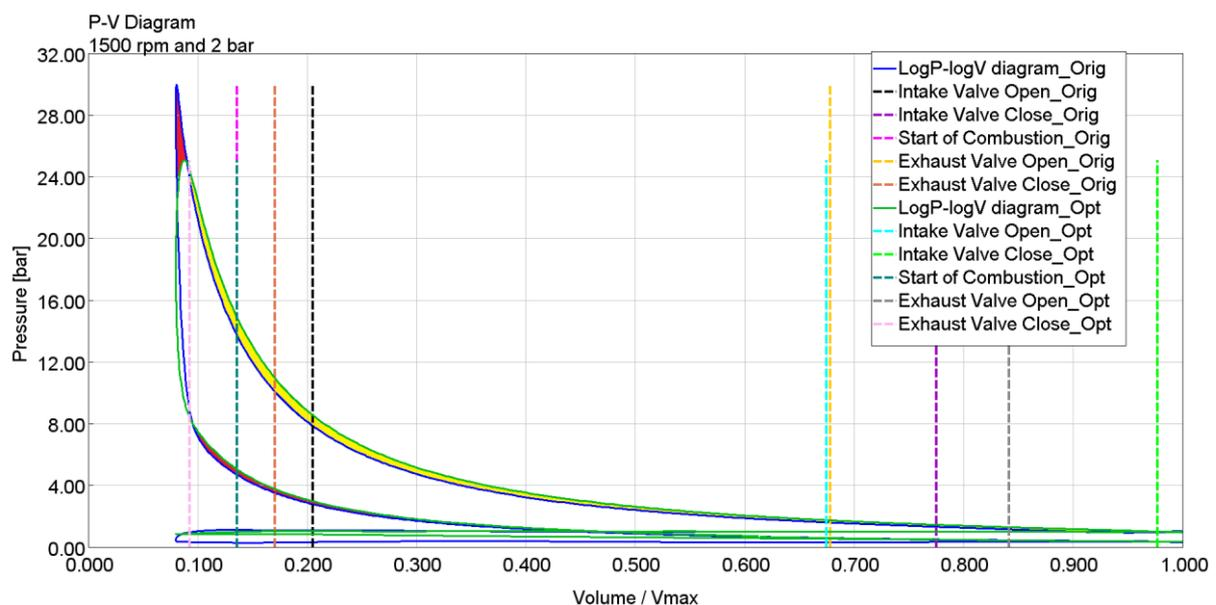
**Figure 6: P-V diagram of the engine before and after optimization at 1500 rpm and 2 bar.**
