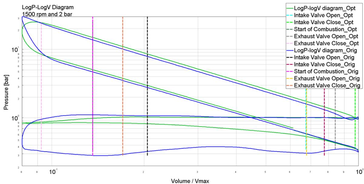
**Figure 7: log(p)-log(V) diagram of the engine before and after optimization at 1500 rpm and 2 bar.**
