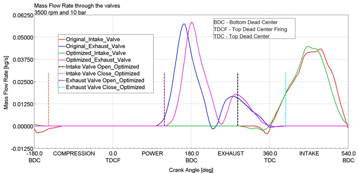
**Figure 9: Graphic of the mass flow through the intake and exhaust valves before and after optimization at 3500 RPM and 10 bar.**
