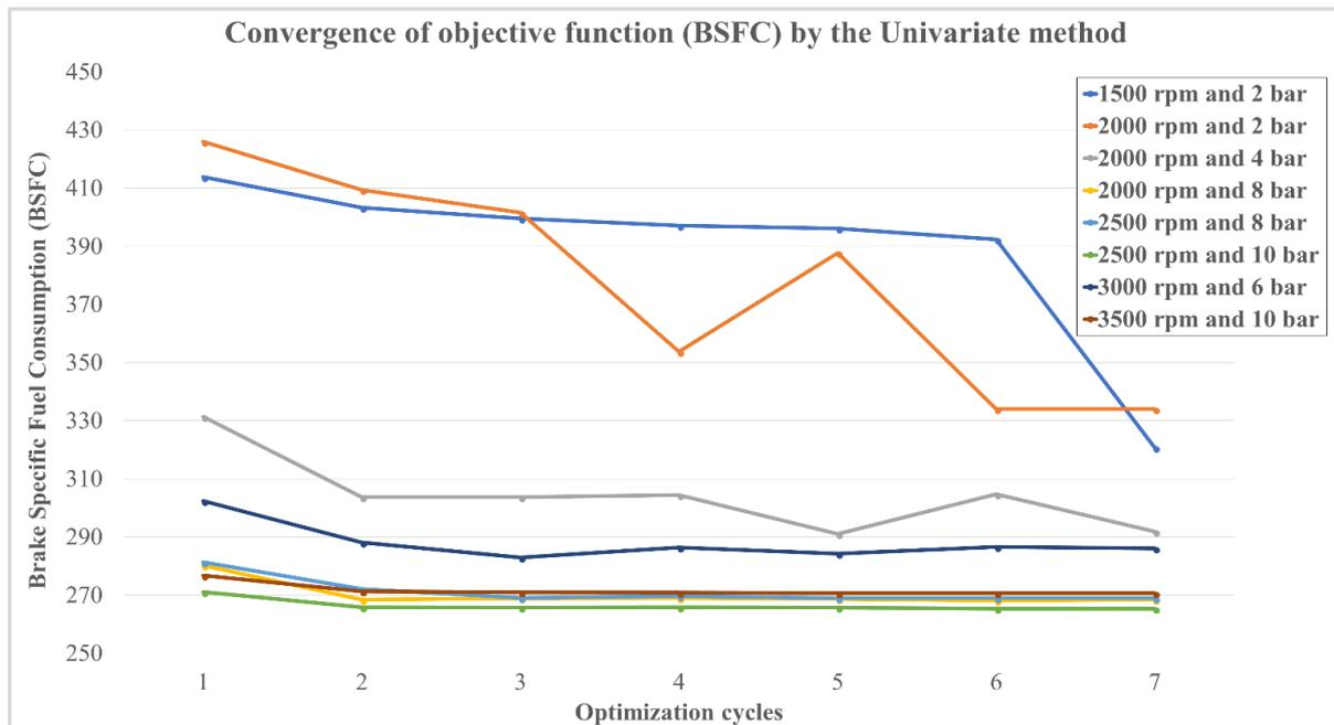
**Figure 2: Specific fuel consumption obtained during the optimization step for the selected operating conditions by the Univariate method.**
