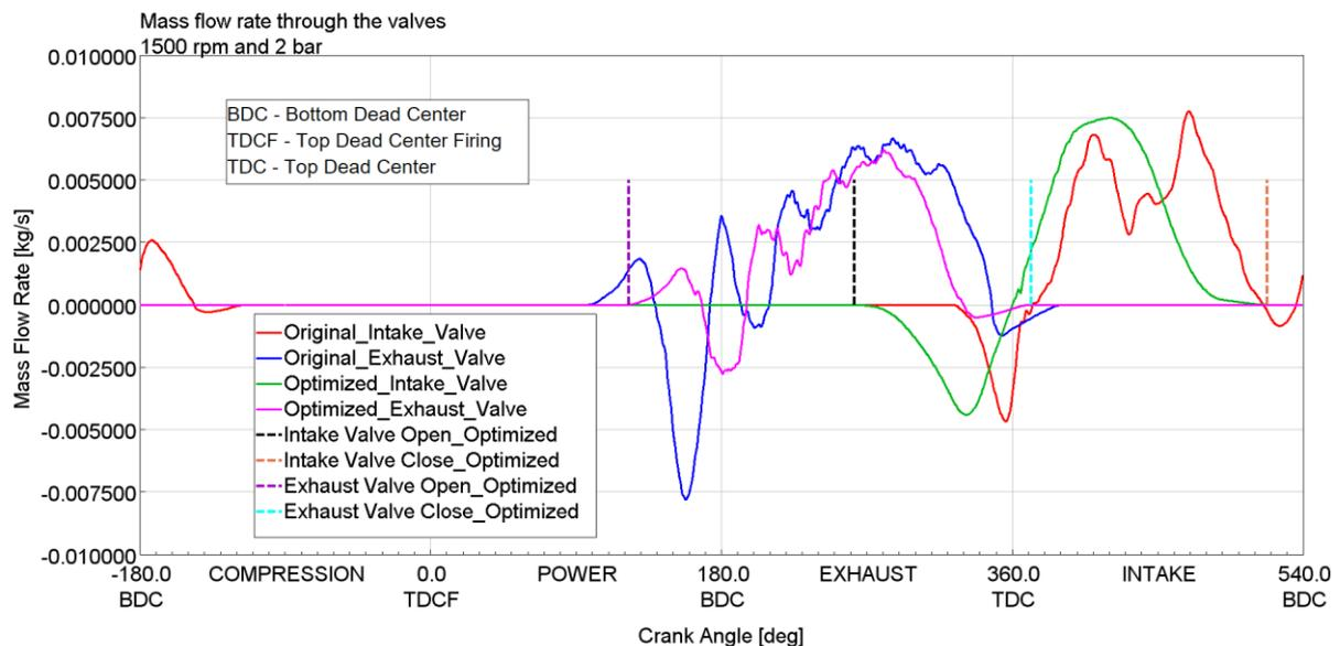
**Figure 5: Mass flow through the intake and exhaust valves before and after optimization at 1500 rpm and 2 bar.**
