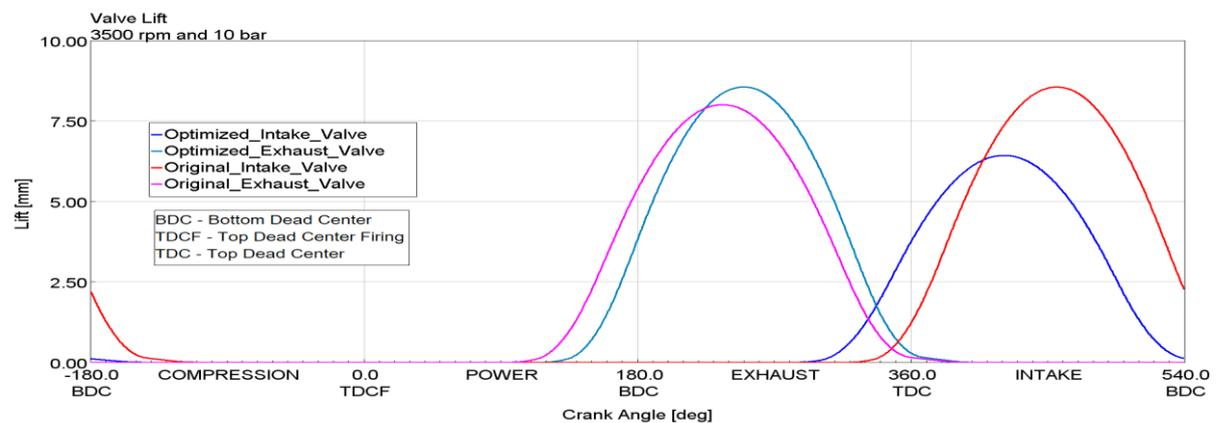
**Figure 8: Valve lift curves before and after optimization for operation at 3500 RPM and 10 bar.**
