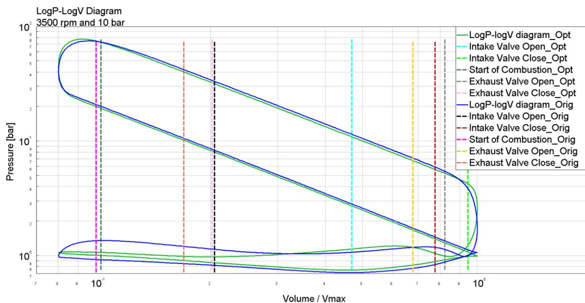
**Figure 10: log(p)-log(V) diagram of the engine before and after optimization at 3500 rpm and 10 bar.**
