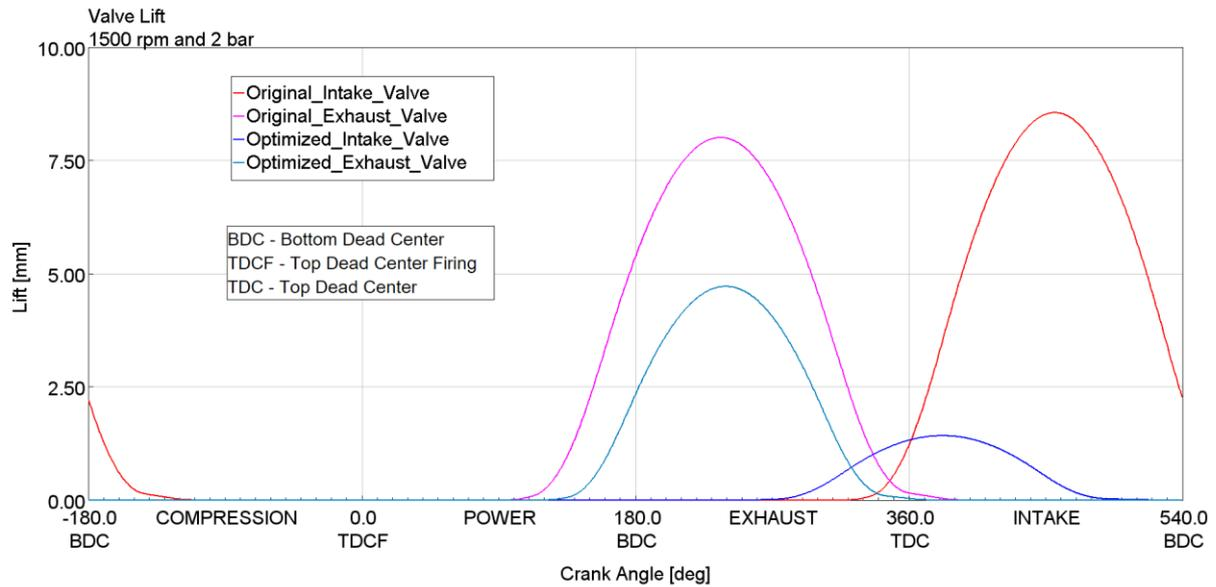
**Figure 4: Valve lift curves before and after optimization for operation at 1500 rpm and 2 bar.**
