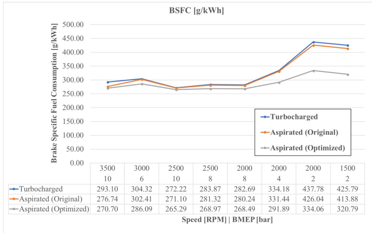
**Figure 3: Specific fuel consumption for the turbocharged model, aspirated engine model with the original cam profile and the aspirated engine model with the optimized cam profile.**
