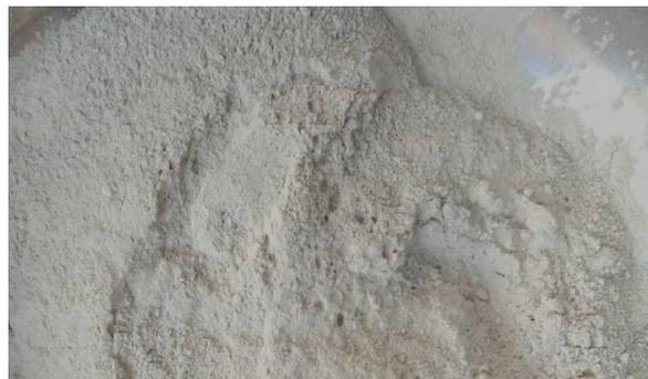
**Figure 3.3: Show the bentonite used as binding agent of the ores.**
