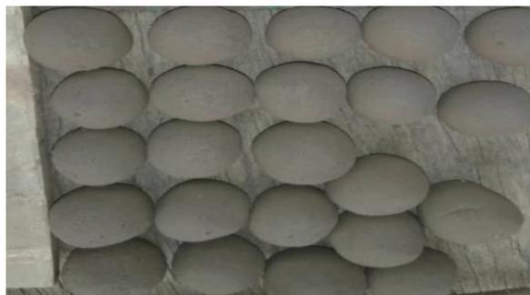
**Figure 3.4: Shows some resultant pellets from Itakpe Iron ore,**
