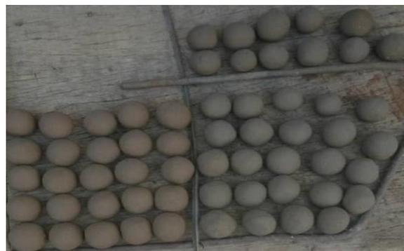
**Figure 3.6: Shows how some resultant pellets for both Itakpe and Agbaja iron ores were dried in the normal atmospheric which is known as green pellets**
