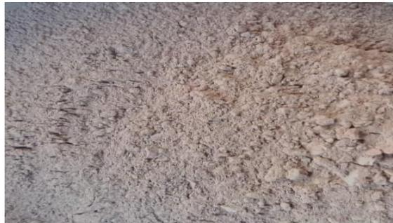
**Figure 2.7: Shows the crushed Itakpe Iron ore prior to pulverization.**
