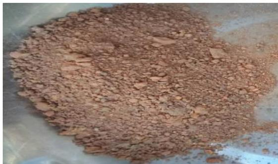
**Figure 2.8: Shows the crushed Agbaja Iron ore prior to pulverization.**
