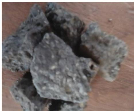
**Figure 2: 5 Shows the Metallurgical Coking Coal after being used as reducing agent.**
