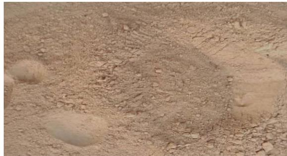
**Figure 3.2: Shows the pulverized Agbaja Iron ore.**
