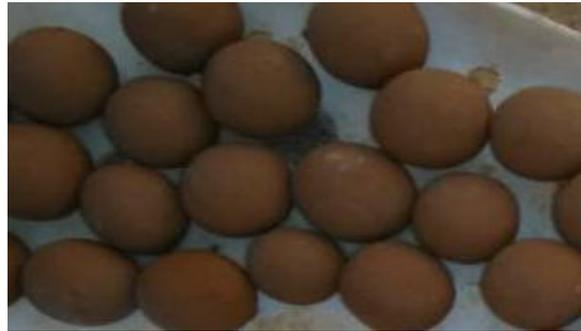
**Figure 3.5: Shows some resultant pellets from Agbaja Iron ore.**
