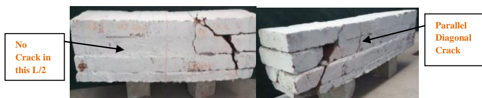
Fig. 8: Failure in TRBWCL2 - Front and Rear view.
