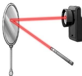
Figure 5: A laser beam has been reflected by the mirror (placed at the left from the laser) and acts with an electromagnetic radiation pressure on the mirror directed
