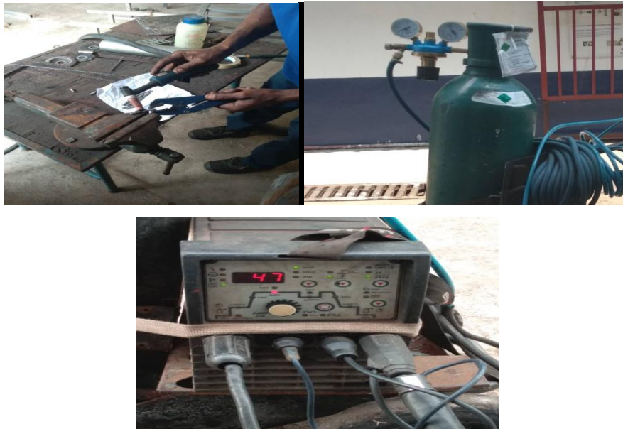
Figure 2.1: welded sample. Figure 2.2: TIG shielding gas cylinder. Figure 2.3: TIG welding machine
