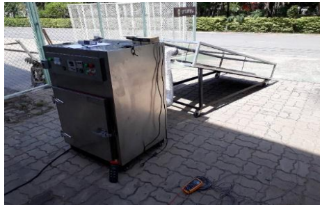
Fig. 3: Hybrid solar dryer design and fabrication.
