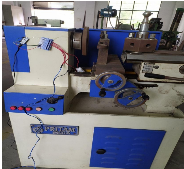
Fig. 7: Relay 3 control the Machine 3 with ESP8266 Microcontroller.
