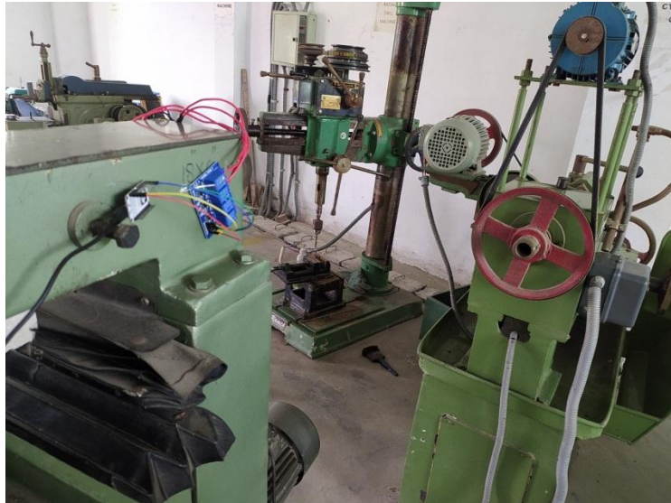
Fig. 2: Shows the implementation of Relay and ESP8266 on Machines.
