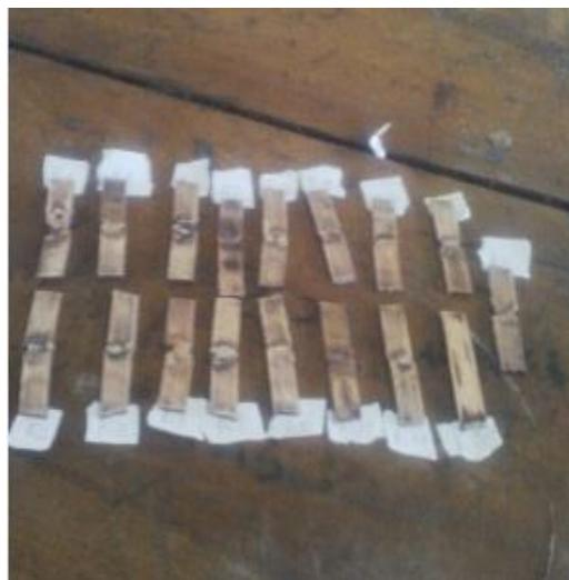
**Figure 1: Impact welded sample.**
