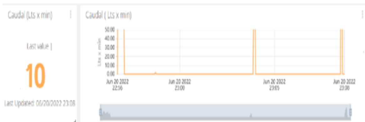
Figure 13: Real Time water flow graph, where the x-axis represents time in hours and the y-axis represents flow in liters per minute (lts x min).
