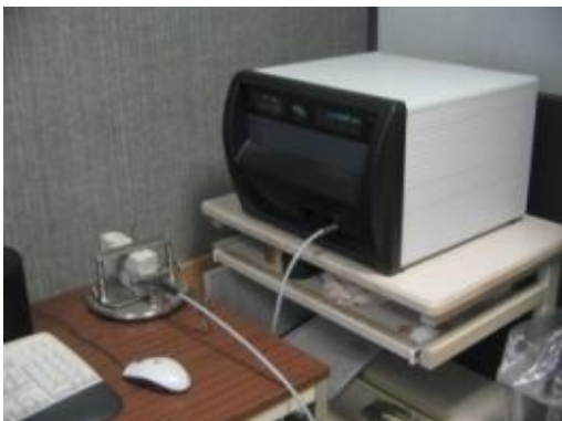
Figure 10: Hot disk measurement process. [2]
