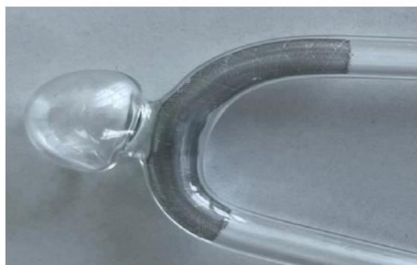
Figure 4: Successful Deployment of Nitinol Flow Diverter into an In-Vitro Neurovascular Simulation Model.
