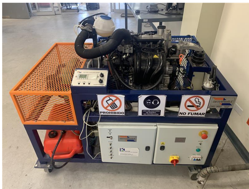
Figure 1: Armfield CM11-KII instrumentation system.
