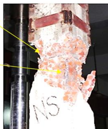
Figure 9 Crushing of the concrete and buckling of the longitudinal reinforcement at the Column NS2.
