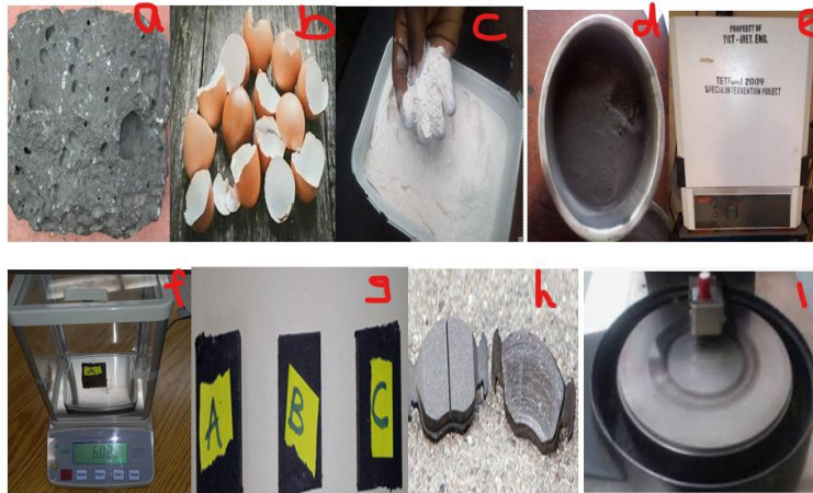
Figure 1: (a) basalt (b) eggshells powder (c) eggshells powder (d) carbonized eggshells powder (e) heat treatment furnace (f) digital weighing samples (g) produced sample (h) break lining (i) wear.
