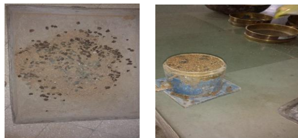
Figure 3: a.) (RAP+virgin aggregate+Fine sand) mix and b.) Proctor mould for the mix.
