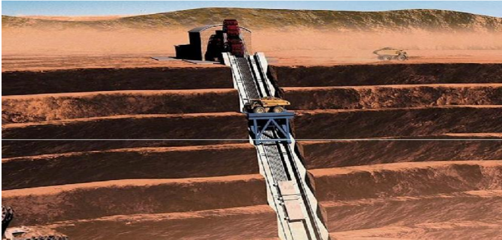
Figure 6: Truck Lift Systems developed by Siemag Tecberg ( http://www.siemag-tecberg.com/infocentre/technical-information/ti_27-trucklift.html ).
