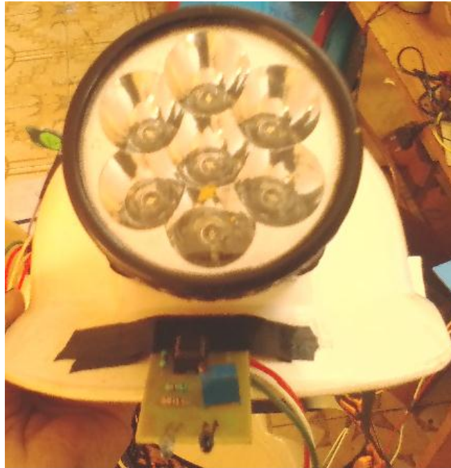
Fig 4: Helmet with IR sensor in the front.
