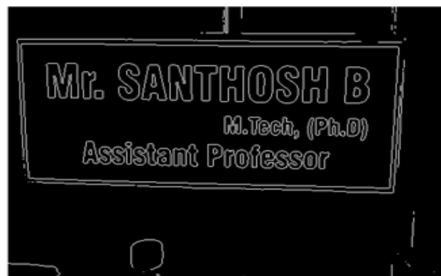
Figure 10: Sobel edge detected image
