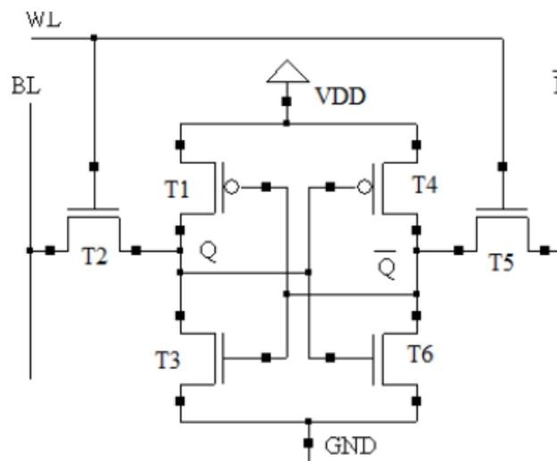
**Fig. 1.1: Circuit diagram of SRAM.**
