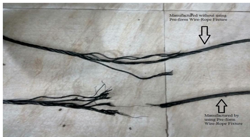
Fig: Wire ropes after testing.
