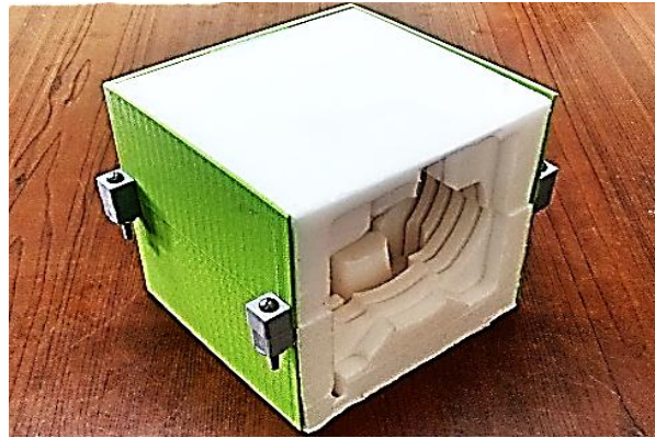
Figure 5: Silicone rubber molds to obtain wax patterns.
