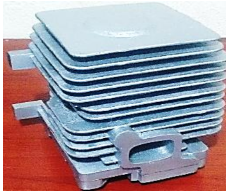
Figure 8: Metallic motor block manufactured by vacuum assisted casting.
