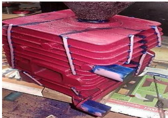
Figure 7: Wax motors block totally assembly.
