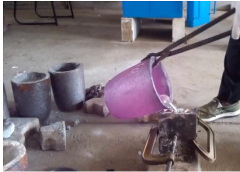
Figure h: Pouring of molten metal into mould box.
