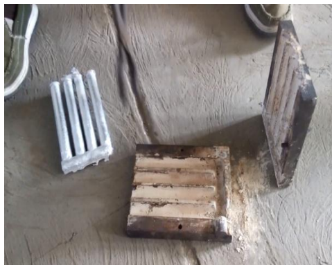
Figure i: opening die Removal of composite from mould box.
