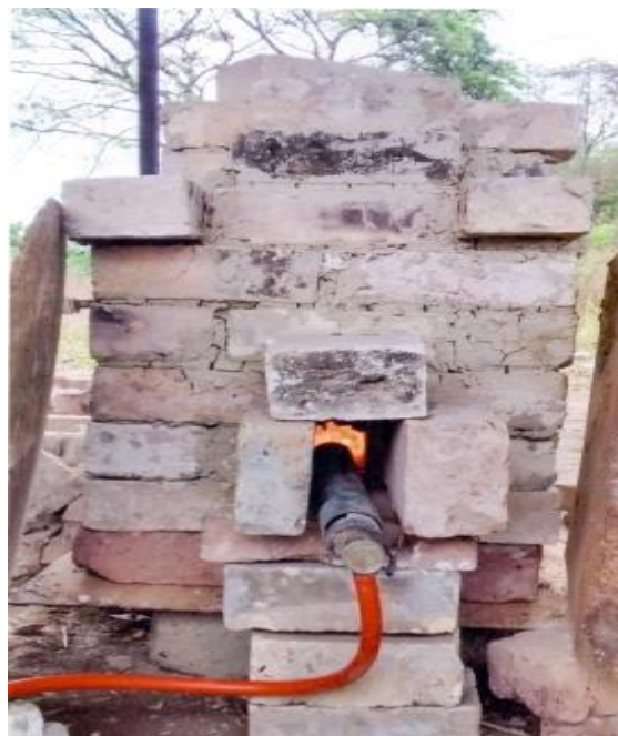
Fig 12: Furnace experimental set-up (Carbonization).
