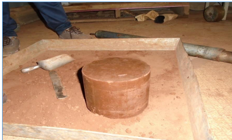
Figure 2.6: Typical compacted soil sample.
