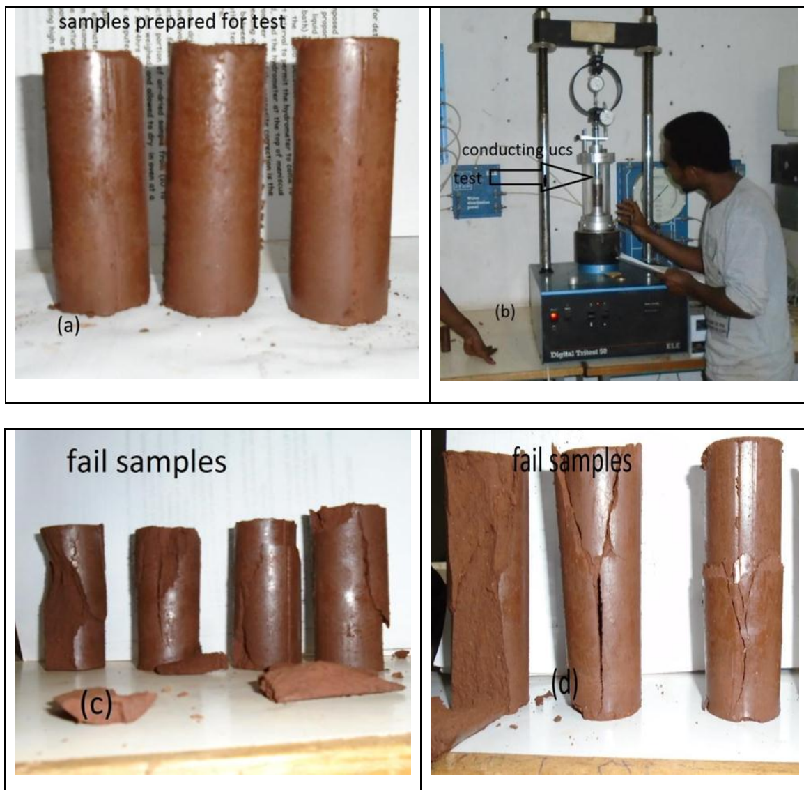
Figure 2.7: Samples prepared for UCS, and typical failure patterns.
