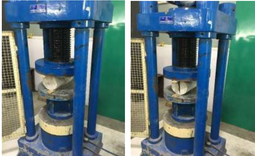
Fig 5: Split tensile strength on cylinder.
