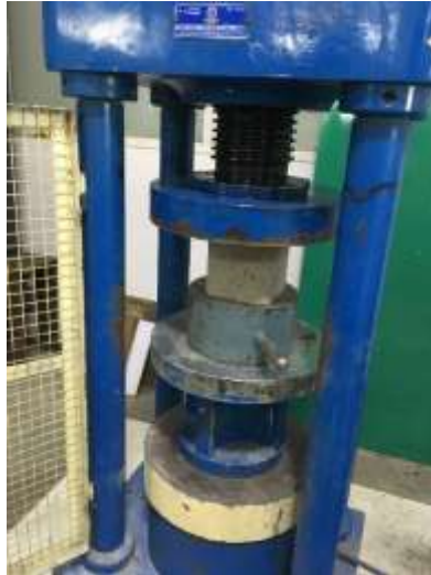
Fig 2: Compression strength on cube.
