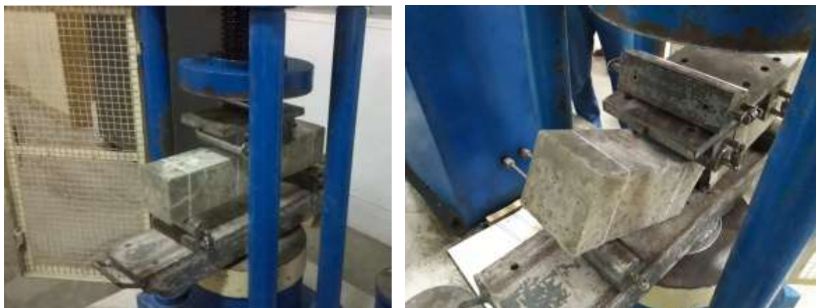
Fig 8: Flexural strengths on Beam.
