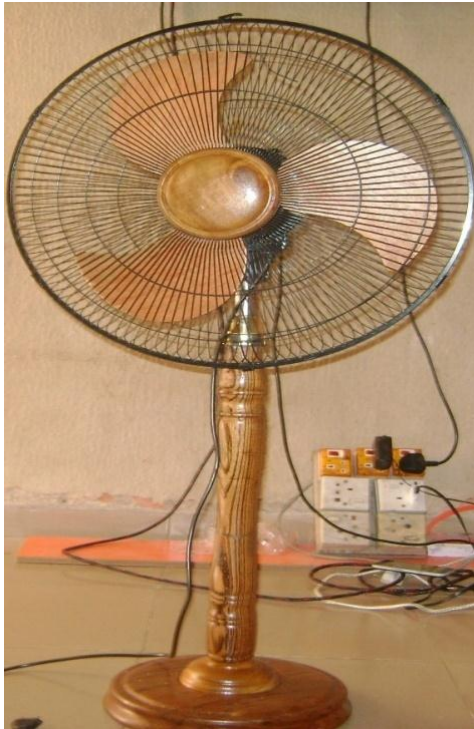
Figure 3: Fan with Blade Diameter, 282.5 mm.
