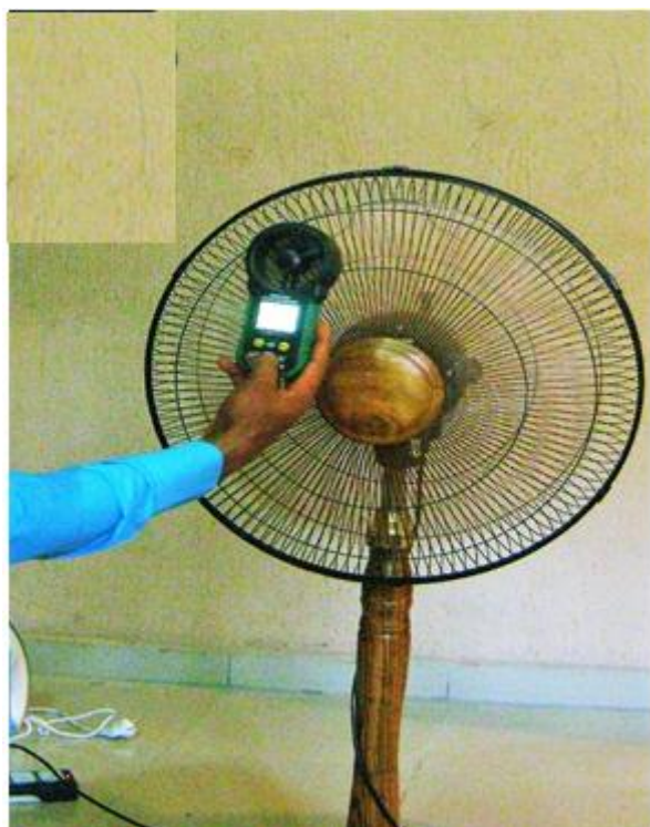
Figure 7: Positioning the Anemometer.
