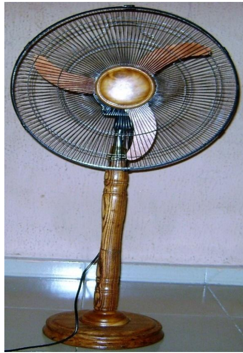
Figure 6: Fan Blade Diameter, 240 mm.
