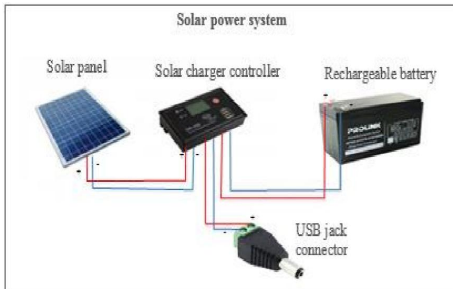
Fig. 2: Solar power system.
