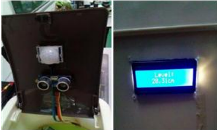
Fig. 7: Sensors attached at the waste bin lid not close an error message will be displayed at the LCD.
