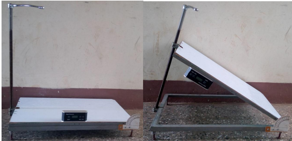
Figure 4: Manufactured Inclino-Tribometer used.
