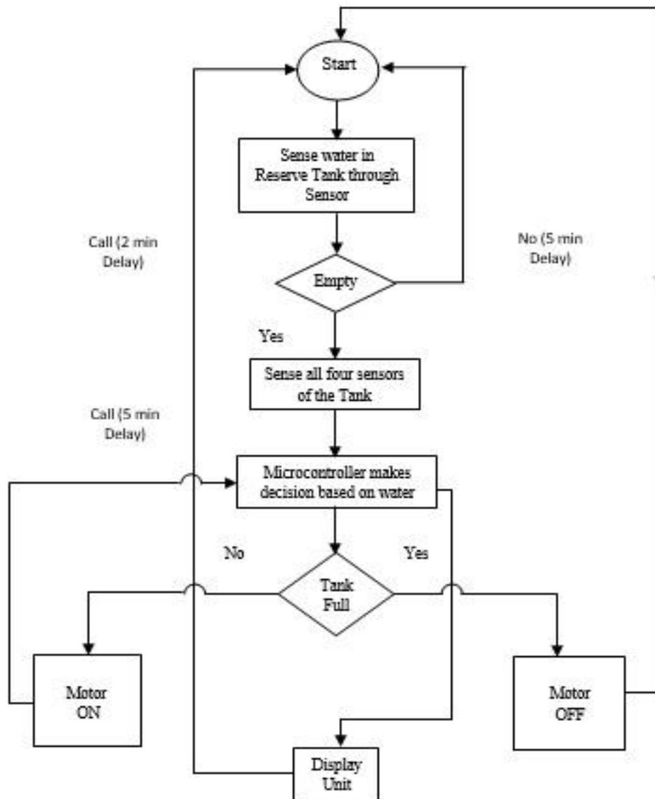
To make the system more easier microcontroller is been used hence the complexity of circuit has been reduced and the design has been simple. Here the water level is sensed by an inverter and input from the sensor unit is taken by a microcontroller. Water pump's action (either ON or OFF) is depended on water status of water tank which is related to input variables. Through a flow chart of whole design is given blow in Fig. 01.
