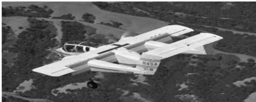
Modified YOV-10A prototype with an integrated rotating cylinder flap, registered N718NA. Courtesy of NASA
