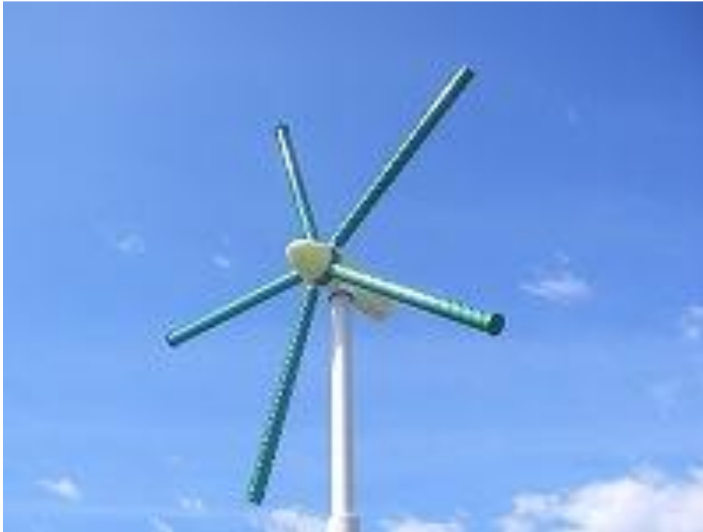
Figure 3.9: Magnus wind turbine operates with 5 rotating cylinders (“MWT-MURAKAMI,” 2010).
