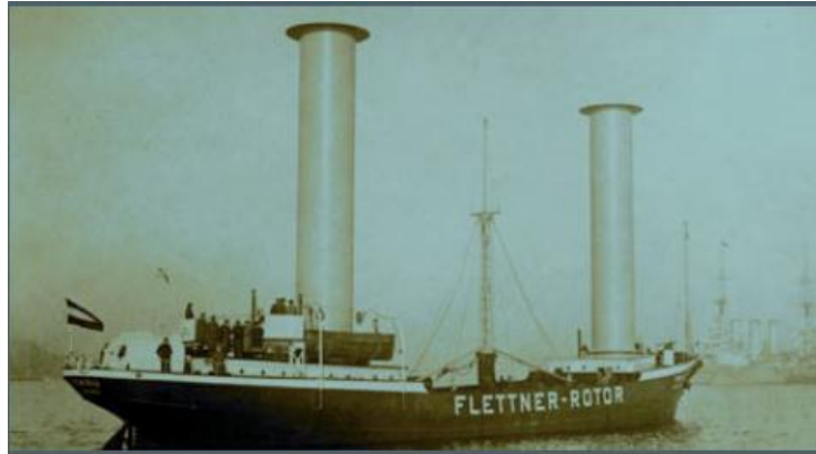
Figure 2.2: Magnus Flettner rotor (Axis & Turbines, 2014).
