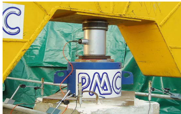
Fig. 3: Example of a Pile load train.
