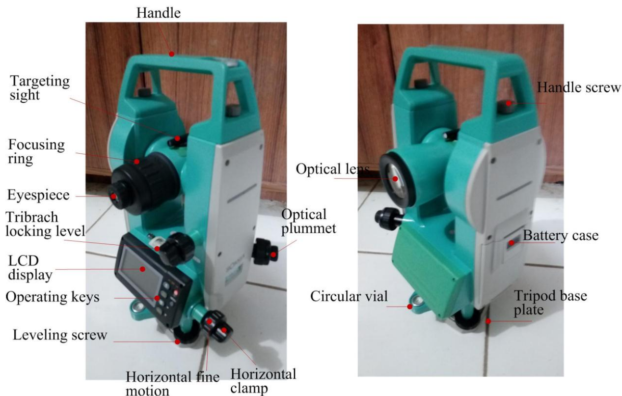
Fig. 3: Diagram of modern theodolite.
