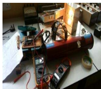
Plate 3(b): Measurement of LDRs' current under the influence of light from
