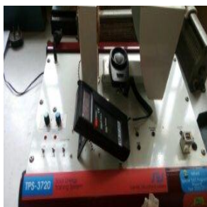
Plate 3(a): Measurement of light intensity using a LUX meter.
