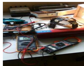
Plate 3(c): Measurement of the voltage across LDRs. Solar Energy Trainer.
