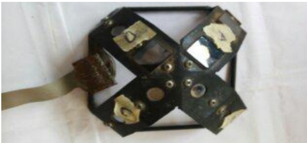
Plate 1: The Four Quadrant Sensor (light dependent resistors)
