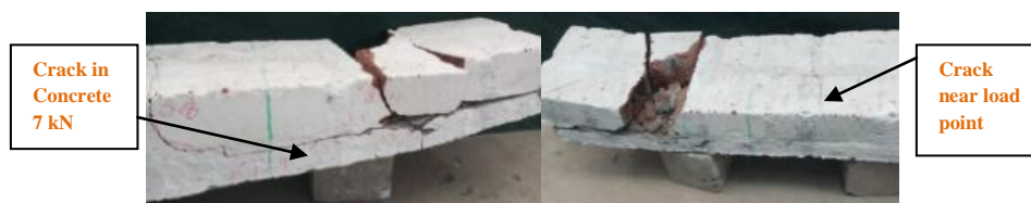
Fig. 7: Failure in TRBWCL1 - Front and Rear view.
