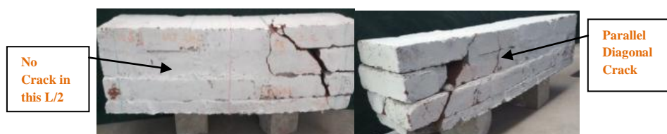
Fig. 8: Failure in TRBWCL2 - Front and Rear view.
