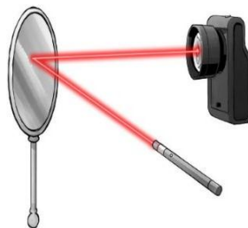
Figure 5: A laser beam has been reflected by the mirror (placed at the left from the laser) and acts with an electromagnetic radiation pressure on the mirror directed
