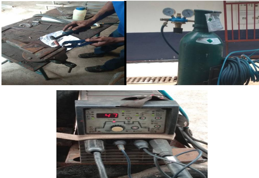
Figure 2.1: welded sample. Figure 2.2: TIG shielding gas cylinder. Figure 2.3: TIG welding machine
