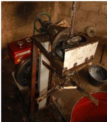
Plate III: Mechanical extractor. Plate IV: Grinding of neem and castor seeds into paste.
