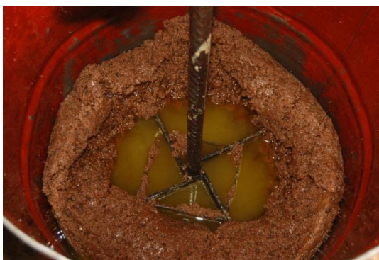
Plate V: Mechanical pressing of neem cake
