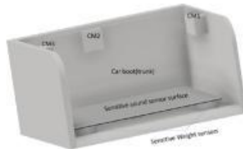
Figure 7: General System installation show positions of sensors for efficient data capture.
