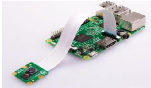
Figure 2: Raspberry Pi and Pi camera interfaced.
