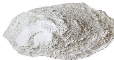
Figure 2b: Cow bone ash after passing through 425µm sieve.
