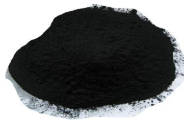
Figure 1b: Coconut shell charcoal after passing through 212 \mu m sieve.
