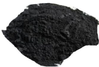
Figure 1a: Coconut shell charcoal before passing through 212 \mu m sieve.
