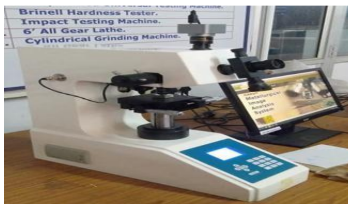
Fig 4: Vicker's Hardness Equipment.
