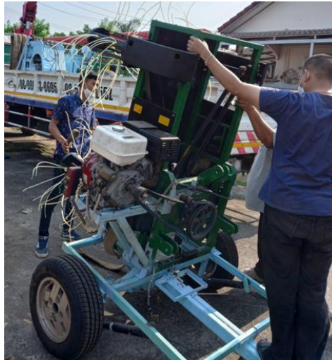
Figure 3: The assembly of the sugarcane leaf cutter on a trailer.
