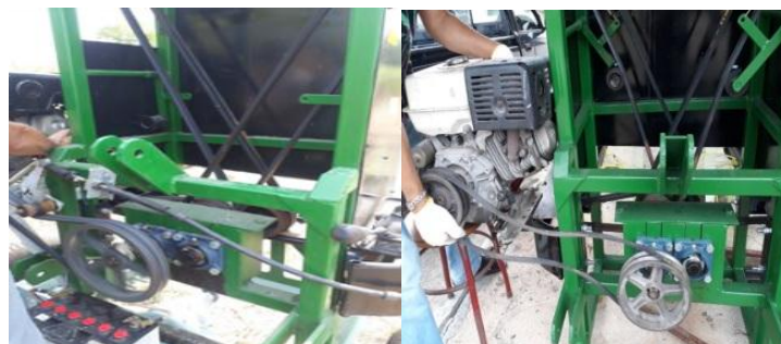
Figure 2: Fabrication of a self-propelled sugar cane leaf cutter.
