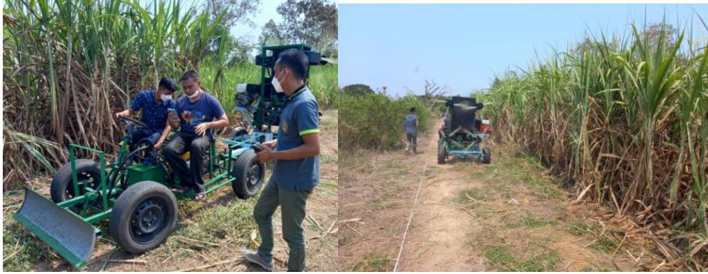
Figure 4: Sugarcane cutter machine field test.
