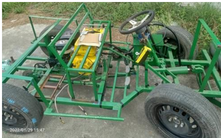
Figure 10: a fabricated small 4-wheel vehicle for agriculture use.
