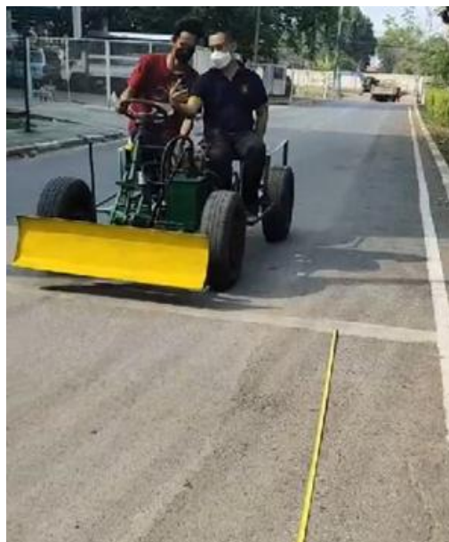
Figure 12: Testing to catch the braking distance.
