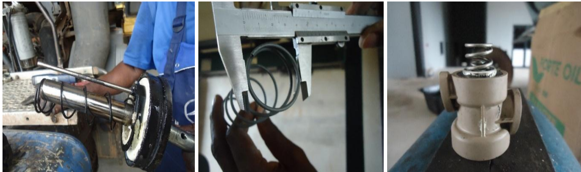
Fig. 3(a): Piston and control valve springs undergoing measurements, (Ndubuisi et al 2022).
