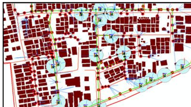
Figure 9: Result of buffering of transformers by 30m.
