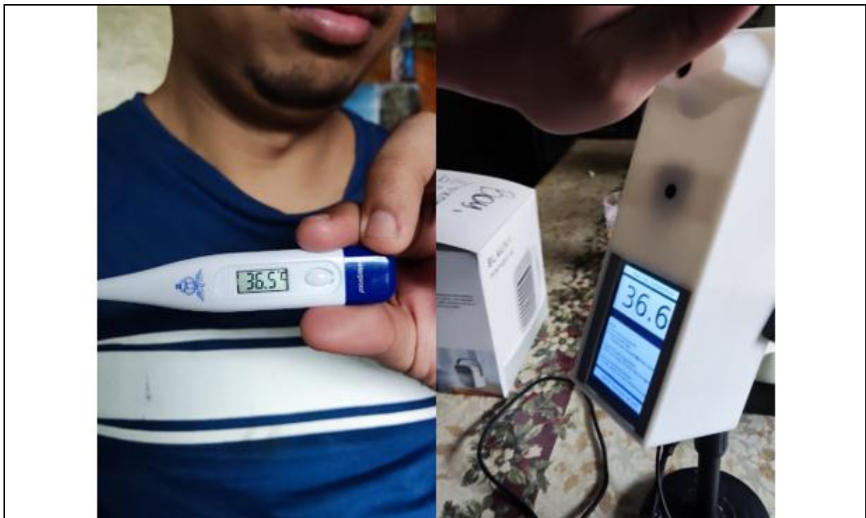
Figure 2: The prototype measuring the temperature (right) and temperature measured using a standard thermometer
