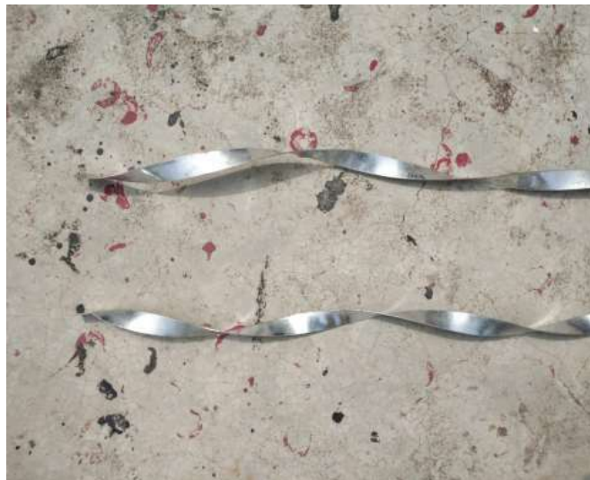
Figure 3: Right Hand and Left Hand Twisted Tape.
