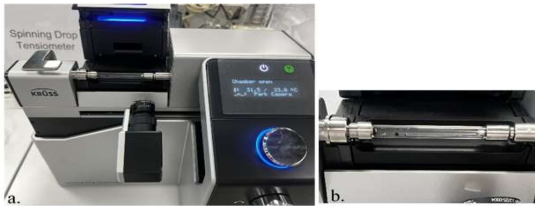
Figure 4: a. KRUSS sinning drop tensiometer
