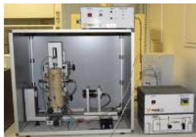
Figure 3: L Teclis Tracker used for IFT and contact angle measurements.
